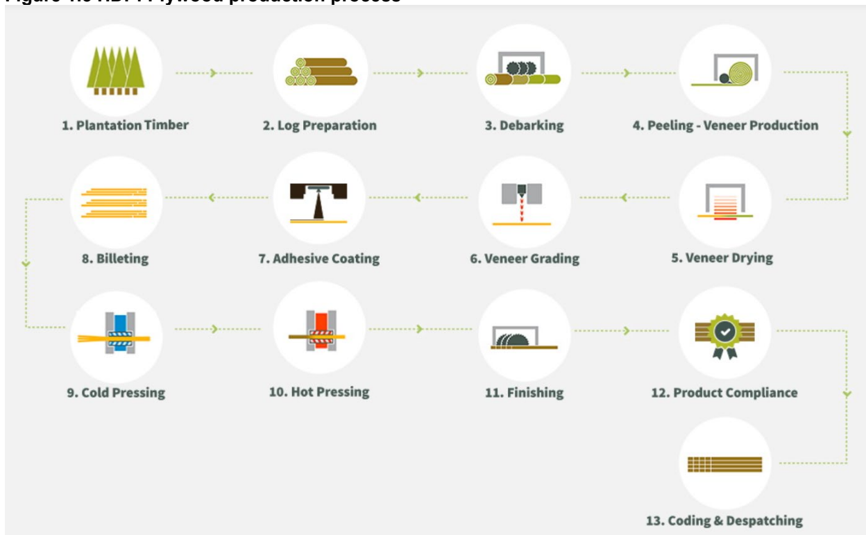
Figure 1.3 HDP: Plywood production process
