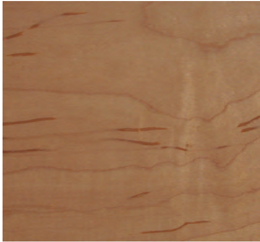
Worm track (Commonly, but incorrectly, referred to as 'vine mark' or 'sugar')
